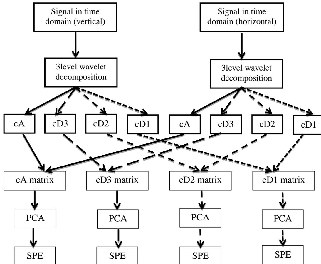
Figure 1. Flow chart of MSPCA\_SPE method [8].
