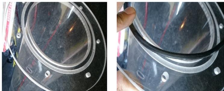
Figure 5. Flanges of heat exchanger.
