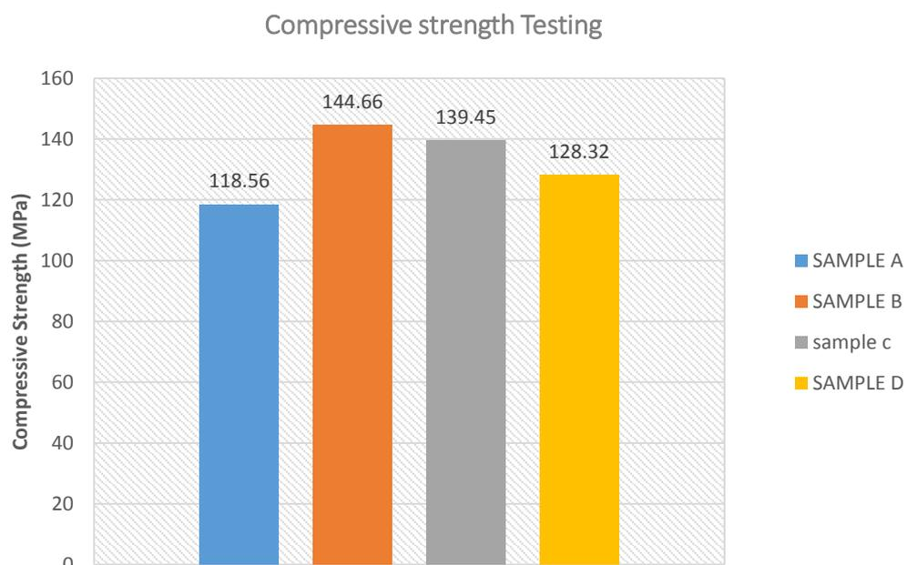
Figure 3. Compressive strength resulting of low carbon steel samples.
