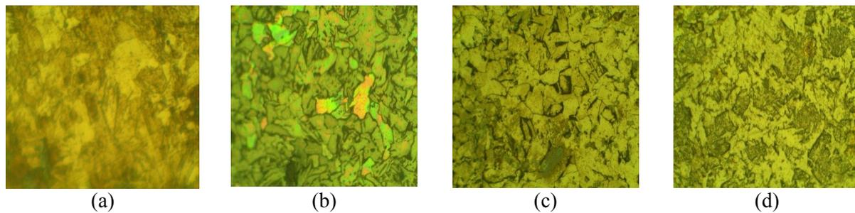
Figure 4. Microstructural examination of (a) as-received sample (b) 25% PE (c) 35% PE (d) 45% PE (at 100x).
