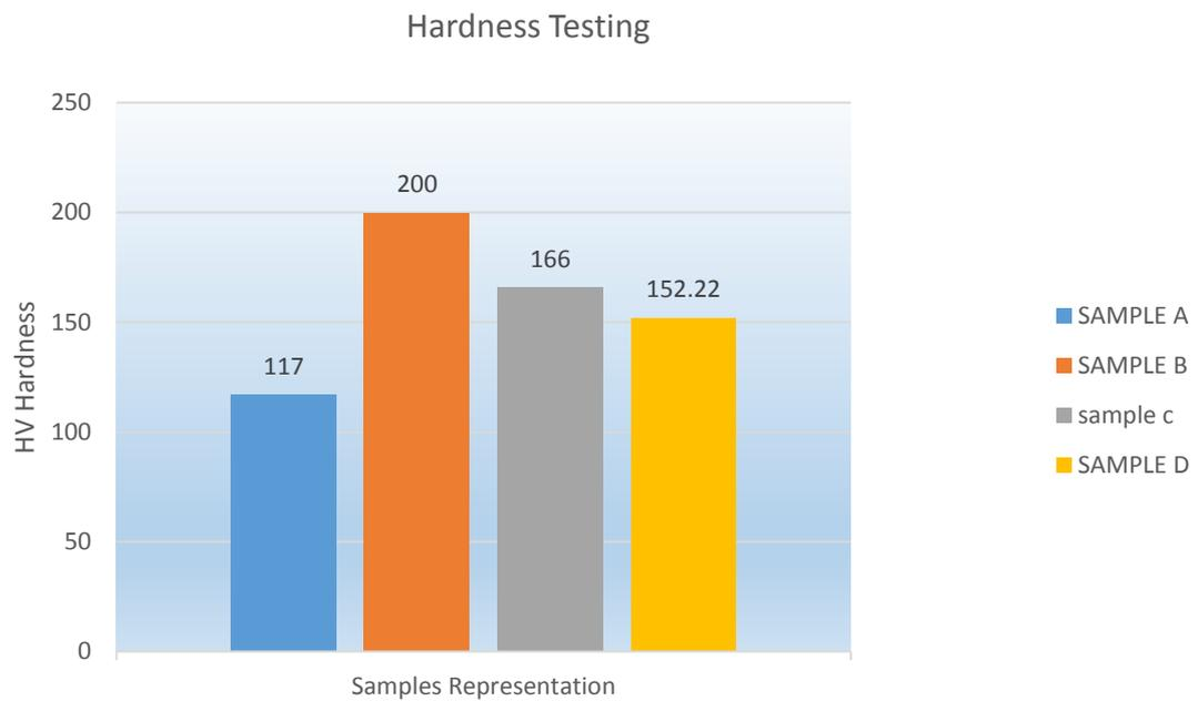
Figure 2. Hardness resulting of low carbon steel samples.
