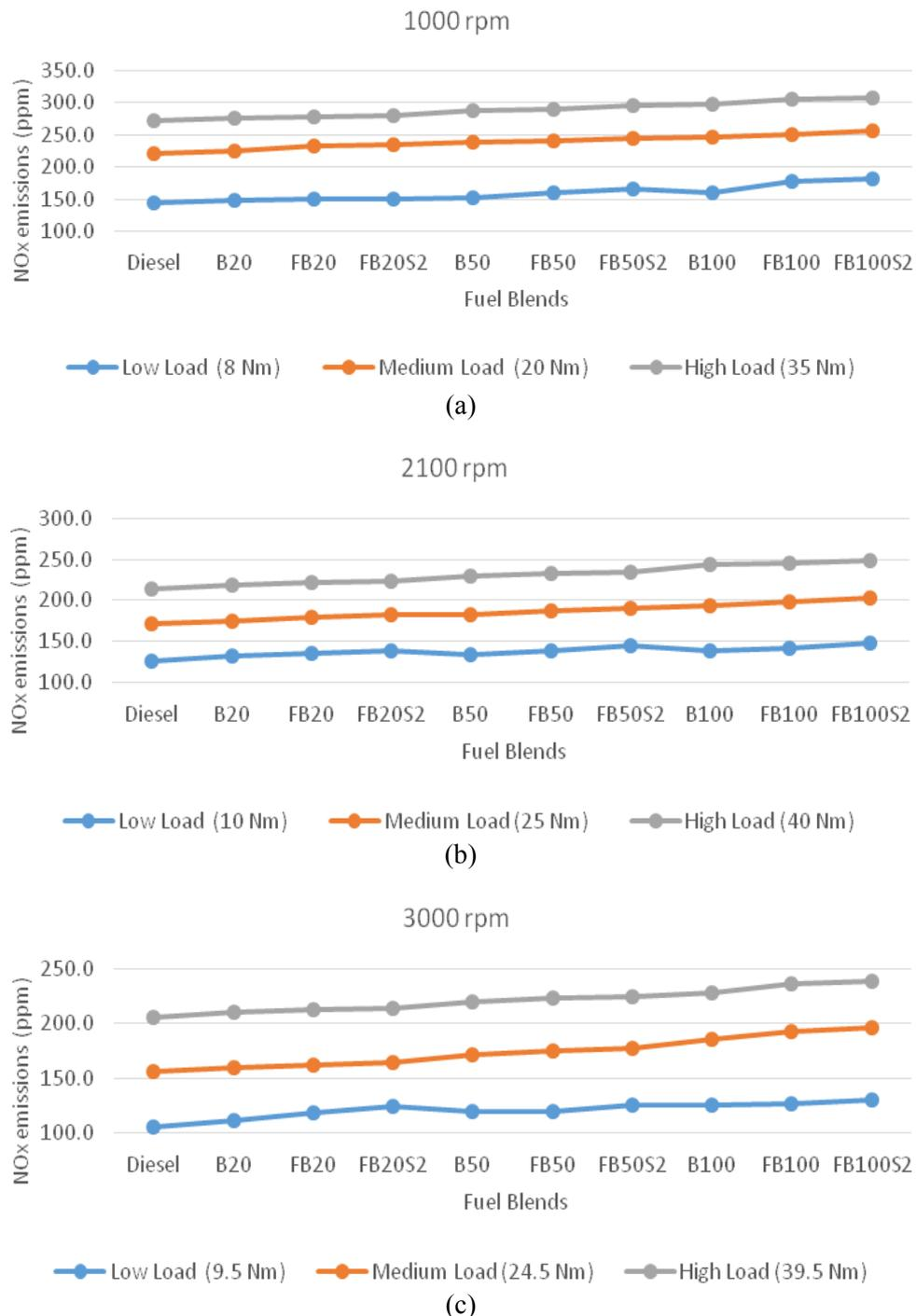
Figure 8. NOx emissions at (a) 1000 rpm (b) 2100 rpm (c) 3000 rpm for different fuel blends under variable engine loads.
