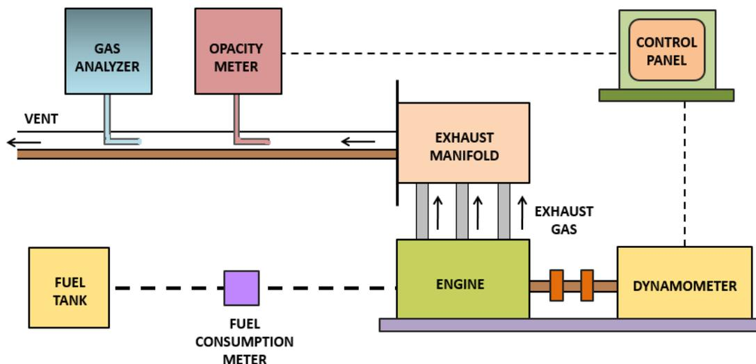
Figure 2. Schematic diagram of diesel engine test setup.
