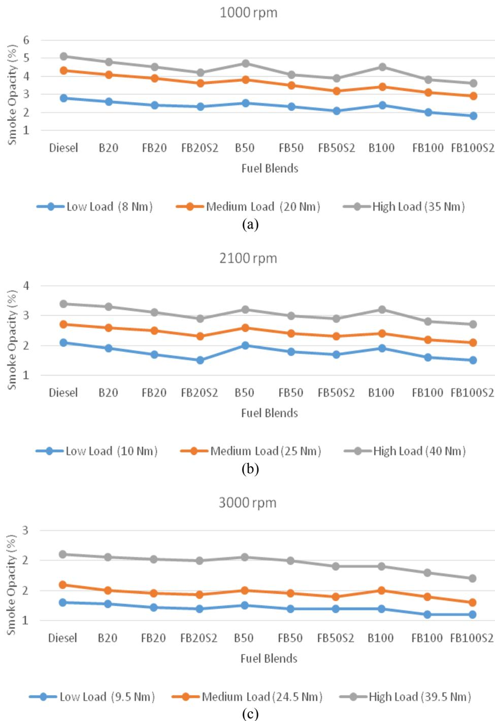
Figure 9. Smoke opacity emissions at (a) 1000 rpm (b) 2100 rpm (c) 3000 rpm for different fuel blends under variable engine loads.
