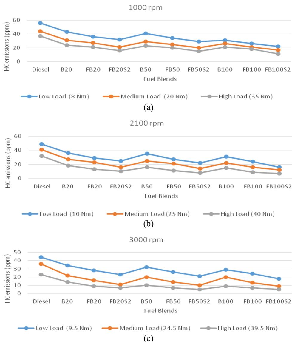
Figure 7. HC emissions at (a) 1000 rpm (b) 2100 rpm (c) 3000 rpm for different fuel blends under variable engine loads.
