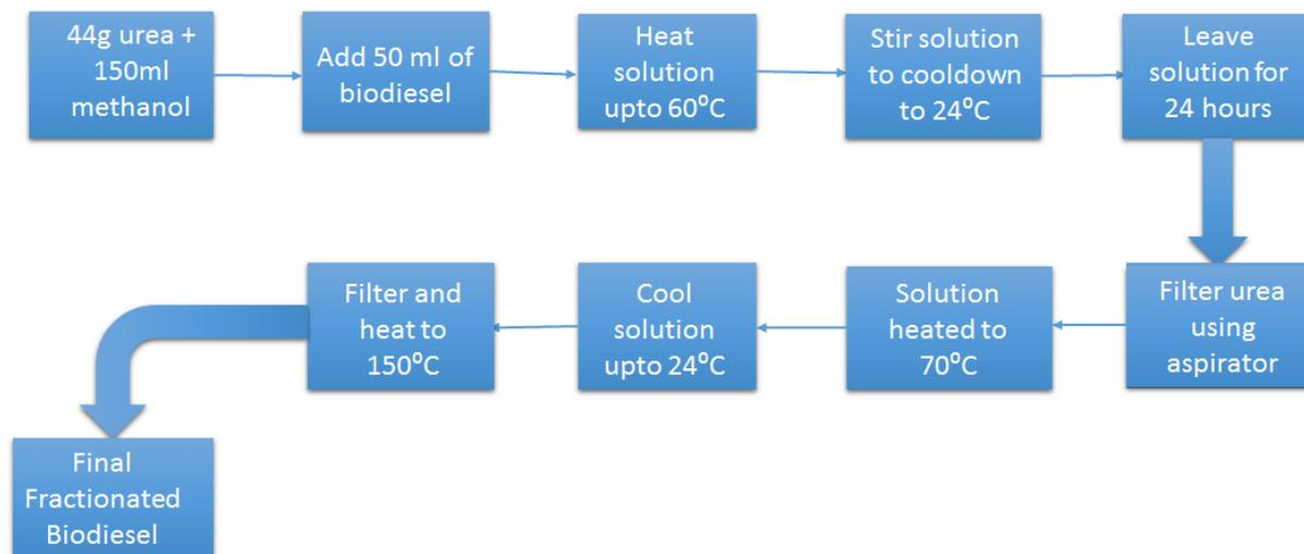
Figure 1. Method of fractionation process.
