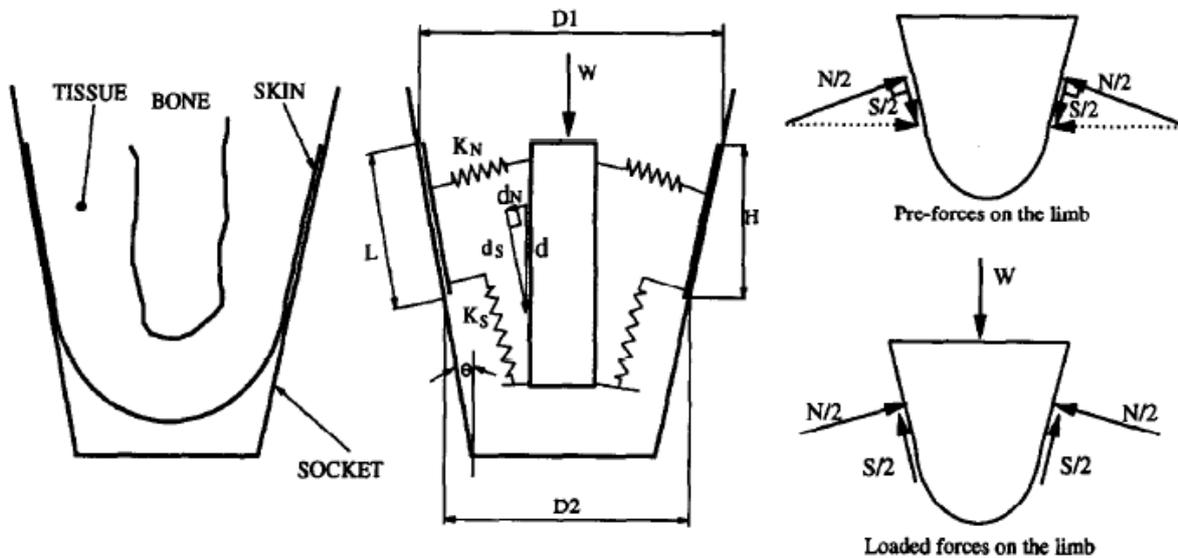
Figure 3. A simplified residual limb model [10].
