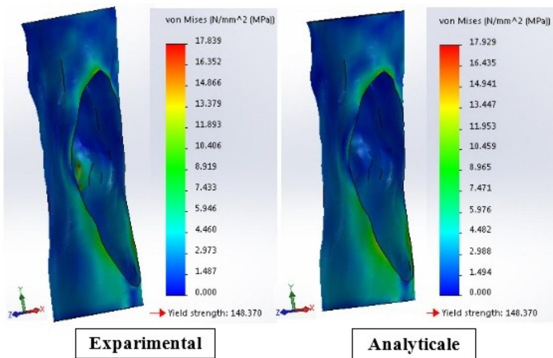
Figure 8. The difference in the Von Mises as contour plot for the two type of simulation.
