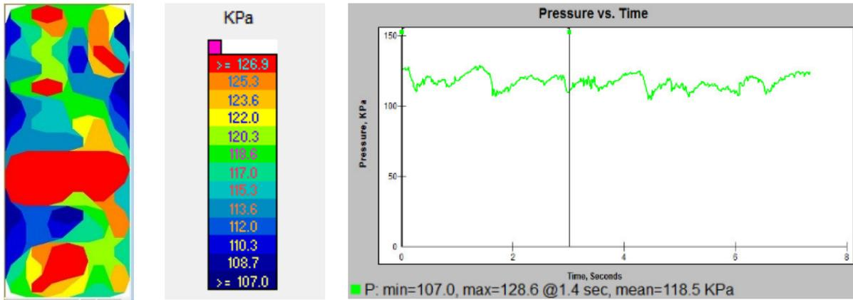
Figure 2. Peak pressure distribution from F-Socket device.
