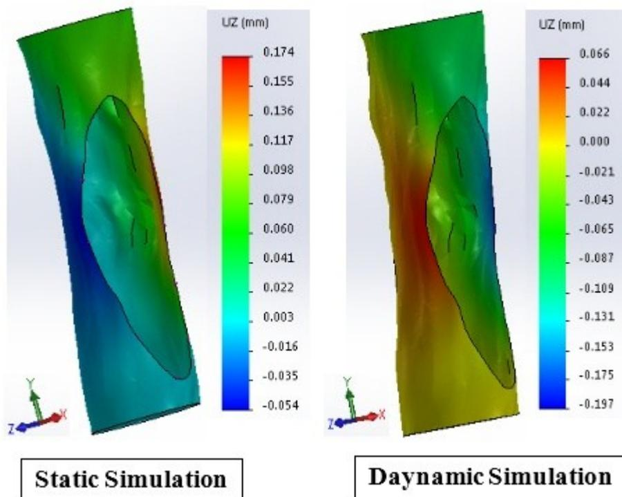
Figure 7. Contour plots of the maximum deformation for the two types of simulation.
