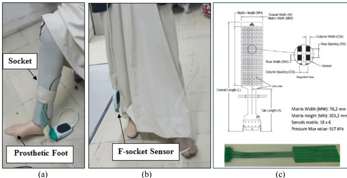
Figure 1. (a, b) The subject during the F-Socket test (c) the shape of the F-socket sensor [5].
