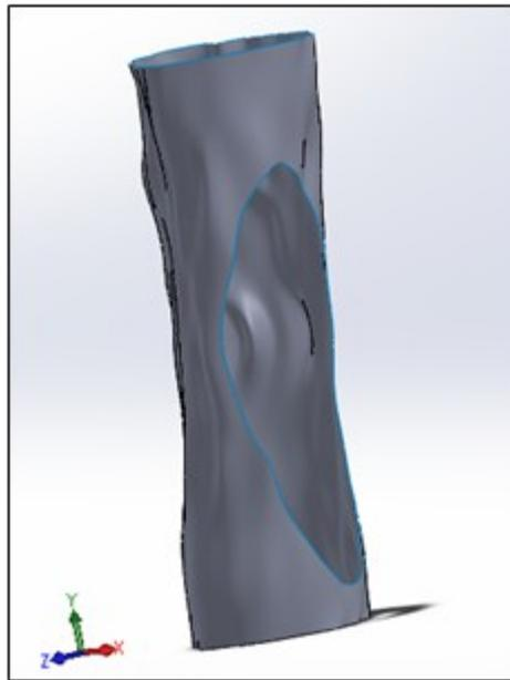
Figure 5. Syme's socket with elliptical cut-out.
