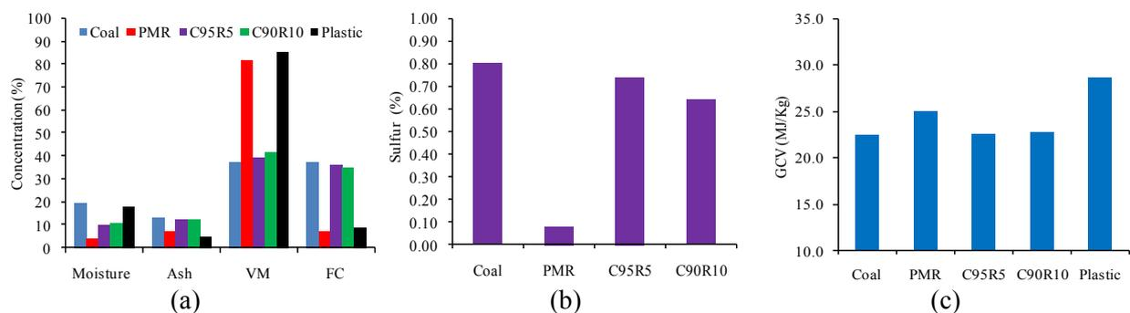
Figure 2. (a) Moisture, ash, volatile matter (VM) and fixed carbon (FC) content; (b) Sulfur content; (c) GCV.
