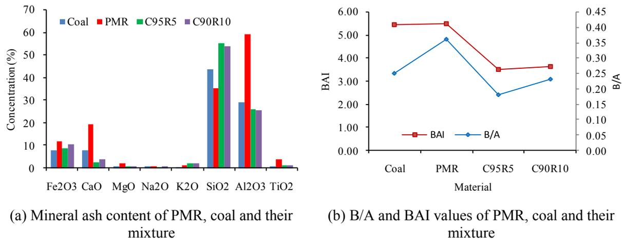
Figure 4. Mineral ash content, B/A and BAI values of PMR, coal and their mixture.
