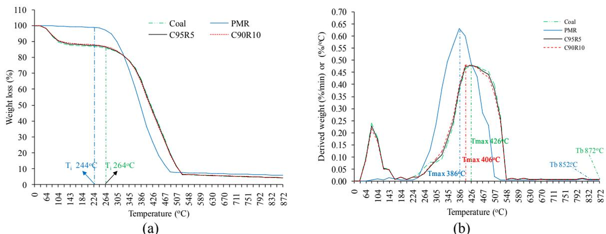
Figure 3. (a) TGA and (b) derived weight in (%/min) or (%/°C) profiles of materials.
