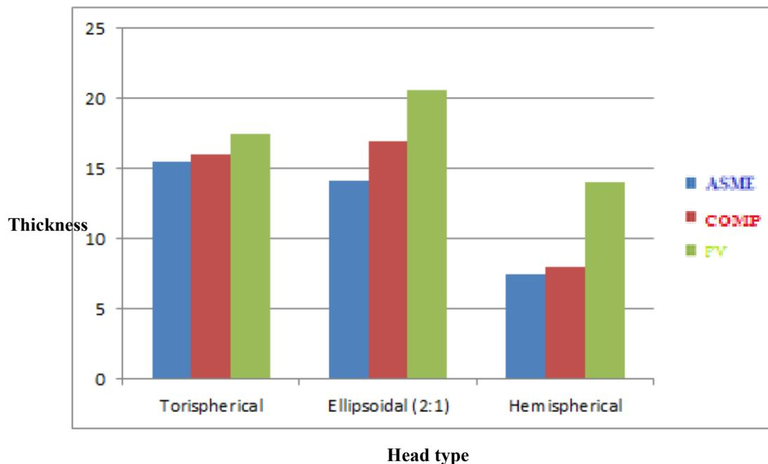
Figure 9. Compression of thicknesses of head obtained by ASME and commercial software.
