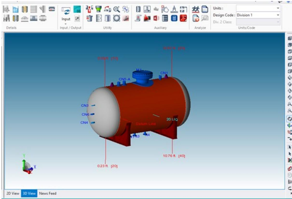
Figure 5. PV Elite wizard window and model building.
