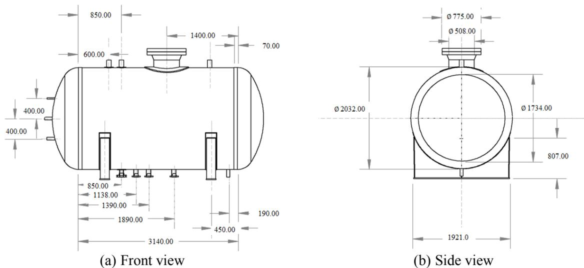
Figure 7. Detailed dimensions of vessel model.
