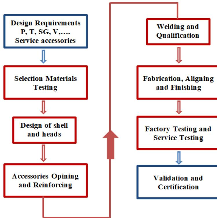
Figure 1. Design steps of pressure vessels.
