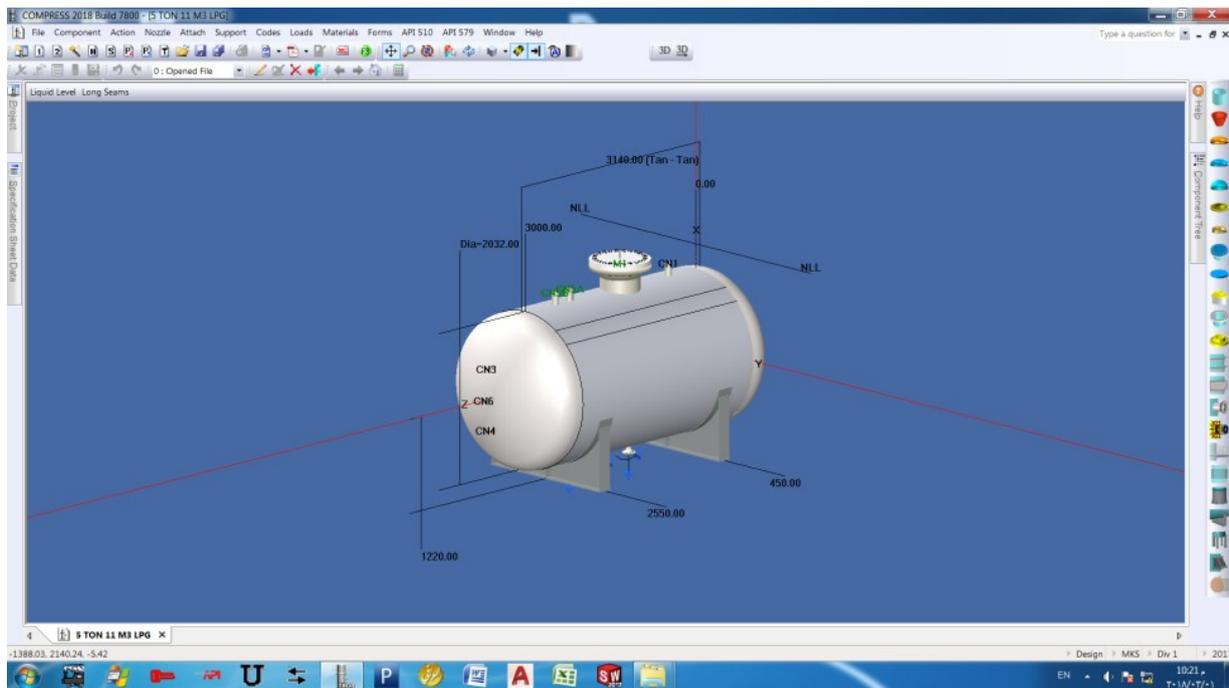
Figure 3. COMPRESS wizard window and model building.
